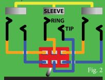
This switch connects the center jack [input] to either the left or right output. You can also use it in reverse to choose between two inputs. The grounds of the three jacks are wired together. That inspired me to buy a sack of DPDT switches and start making my own signal routers, but in stereo. [DPDT stands for "double pole, double throw" — two internal, ganged switches route signals to one of two outputs, or poles.] Figure 1 shows my first project, a simple stereo A/B switch. I connected the
