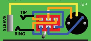
Pin 2 in the MIDI jack [ground/green] is wired to the sleeve of a 3.5mm jack. A DPDT switch toggles Pin 4 [current source/orange] and pin 5 [current sink/blue] between the tip and ring.
