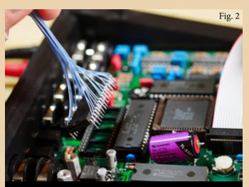
Typically, HR-16 benders remove the voice board and solder wires to the bottom of the chip socket. I used wire-wrap instead.
