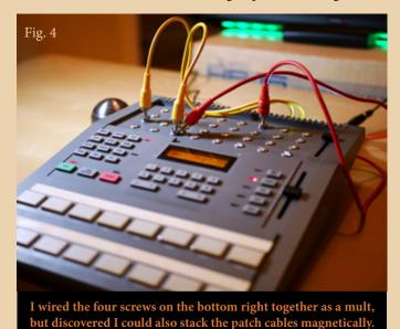
Finally, I made magnetic patch cords by jamming 3/8-inch neodymium ring magnets onto RCA cables. [A 12-pack of ring magnets costs \$5 at Home Depot.] I oriented the magnets to repel each other when facing head-on, which lets me stack plugs by sticking the tip of one plug to the back of the other. [See Figure 4.] The cables are so quick to move that I can easily perform rhythmic effects. Visit Batmosphere.com/hr16 for more hacking tips.
