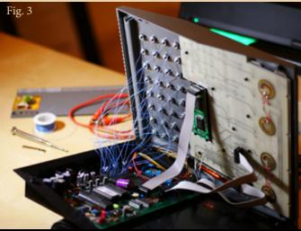
I attached the other end of the wires to #8-32 machine screws with nuts. Notice the four piezo sensors under the drum pads, a clever way Alesis measured how hard you hit.
