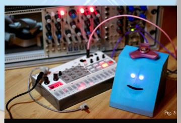
Bolted to a creepy Takada Facebank, my magnetized fidget spinner flashes the purple eyes and sends a 5V pulse proportional to the speed of the spin. See it in action at batmosphere.com/fidget.
